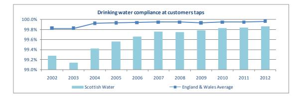
In 2012 we took 153,433 samples at customer taps and tested for 51 different impurities. These tests showed we exceeded the standards in 215 of those samples and mainly in relation to the 8 impurities shown in Figure 5.3.
